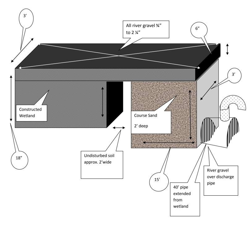
May be in trenches or beds-300 sq ft per bedroom. (45 sq ft) sand filter required following any constructed wetland system
